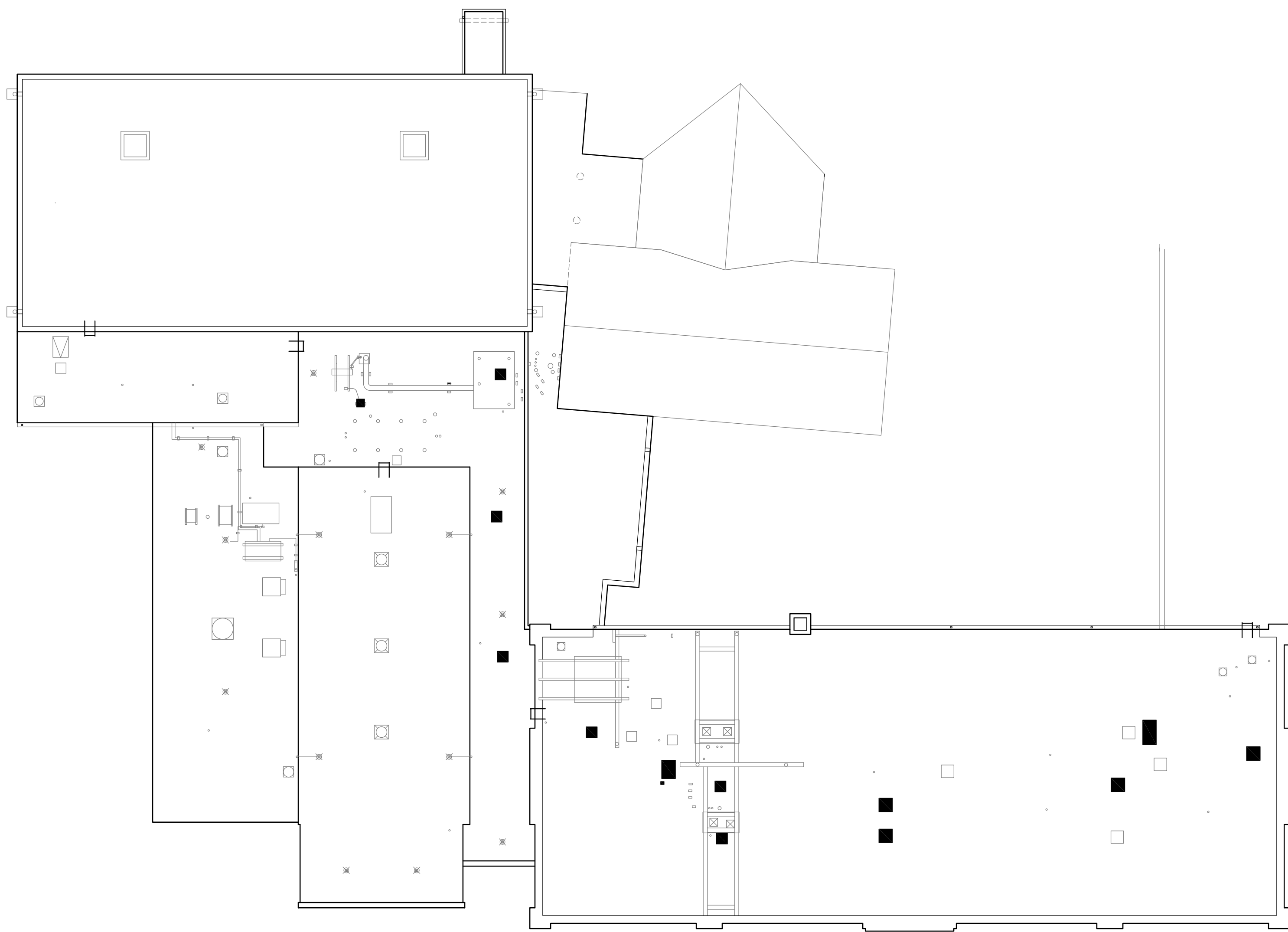
1 DETAIL, CONCEALED STEEL PLATES SCALE: 1/16" = 1' - 0" LOCATIONS ARE SHOWN AS SOLID FILL. SIZE REPRESENTS THE DECK OPENING, NOT THE PLATE SIZE.
