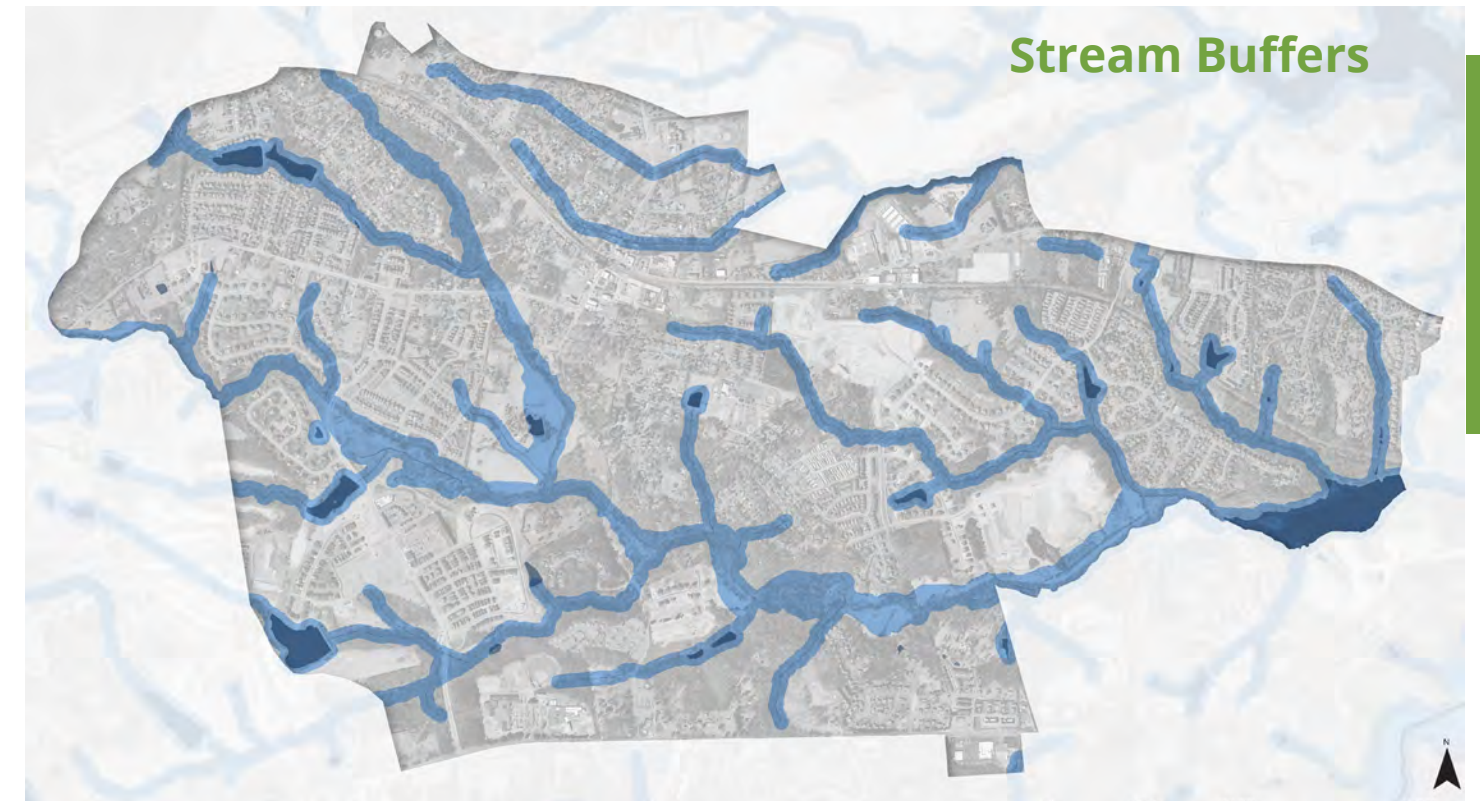
The map above shows stream buffers within the Crozet Development area (transparent blue) and waterbodies (dark blue). Stream buffers are areas of land at or near stream banks and/or nontidal wetlands that provide environmental services, such as improving water quality, or are sensitive to changes that may result in water quality degradation. These areas are regulated by Albemarle County's Water Protection Ordinance, and are often referred to as the "WPO buffer".
